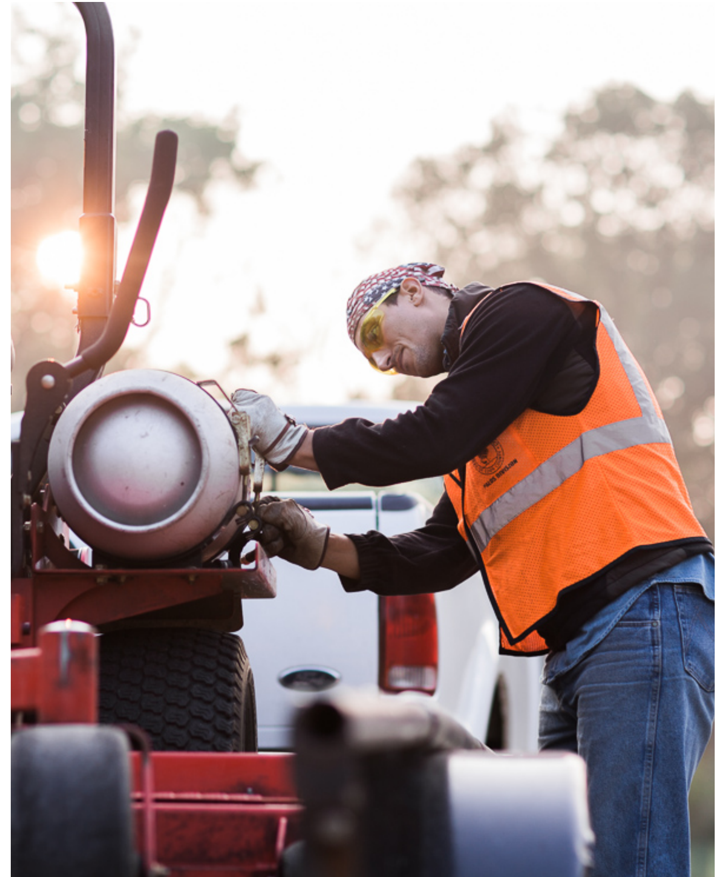
A Forest Preserves employee secures the propane fuel tank on an alternative fuel riding mower. The Forest Preserves introduced propane riding mowers in 2012 while phasing out diesel riding mowers. Using propane riding mowers is one way to reduce carbon emissions and maintain air quality.
